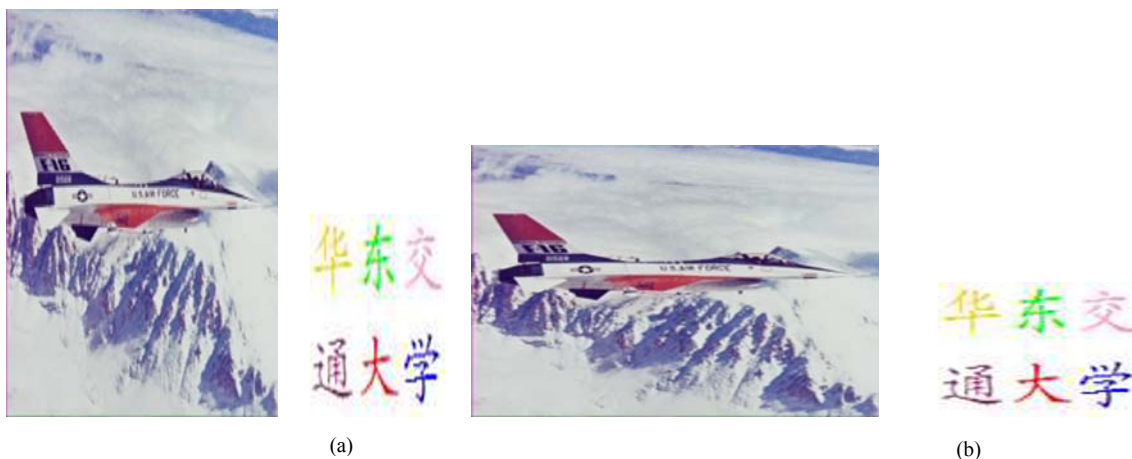
Figure 8. (a) Watermarked image (height stretched to 2 times) and extracted watermark (b) Watermarked image (width stretched to 2 times) and extracted watermark
