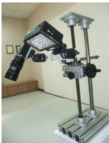
Figure 9. Prototype of scraping guide ways inspection device
