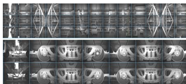
Figure 1. Fifty-three photos from Chinese trouble of freight car detection system.
