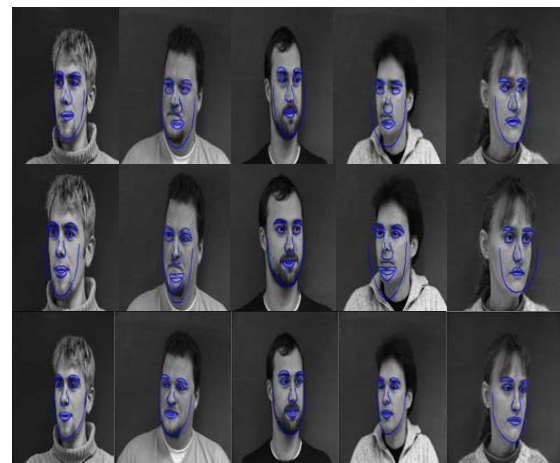
Figure 10. The searching results under pose variation by ASM (first row), ASM+LBP (second row) and the proposed method (third row)
