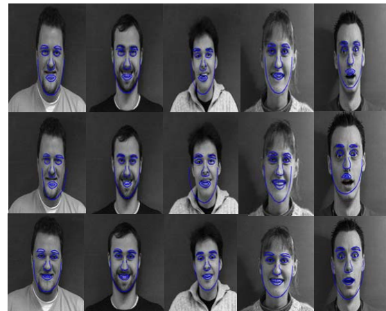
Figure 14. The searching results under expression variation by ASM (first row), ASM+LBP (second row) and the proposed method (third row)
