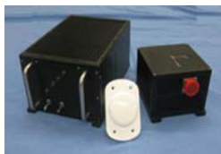
Figure 8. High Precision Fiber Top POS System ( 2.9 kg)
