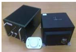
Figure 10. High Precision Laser Top POS System ( 6.5 kg)
