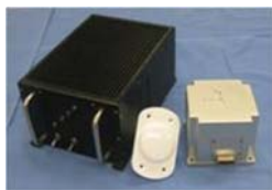
Figure 9. Small Flexible Fiber Top POS System ( 1.5 kg)
