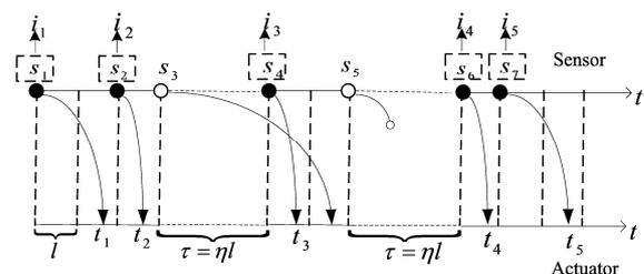
Figure 2. Packet transmission conditions of NCS
