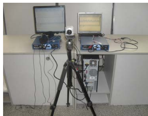
Figure 1. The infrared dynamic image acquisition system and the physiological recording instrument
