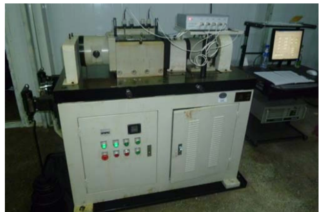
Figure 2. Accelerated bearing life test-ABLT-1A
