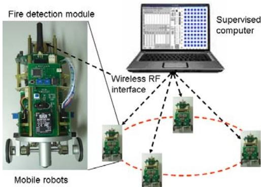
Figure 1. The system architecture and the mobile robot
