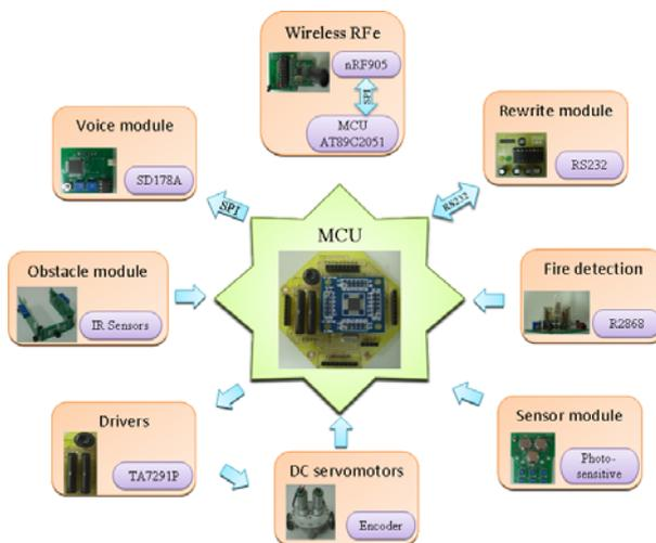
Figure 2. The block diagram of the mobile robot
