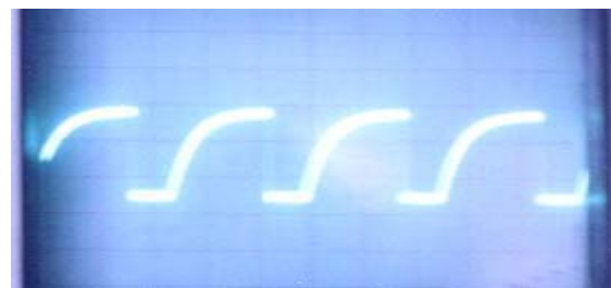
Fig 9a. Pulse generated from opto coupler
