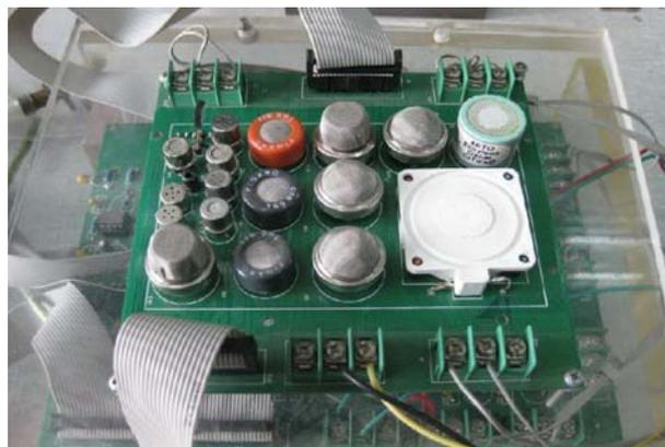
Figure 1 The array of sensors.
