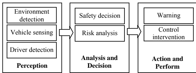
Figure 1. architecture of vehicle anti-collision warning system
