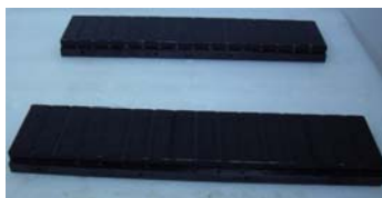
(b) Secondary of unit motor
