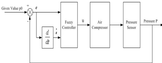
Figure 5. Structure figure of fuzzy control for pressure
