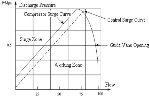
Figure 2. Characteristic curve
