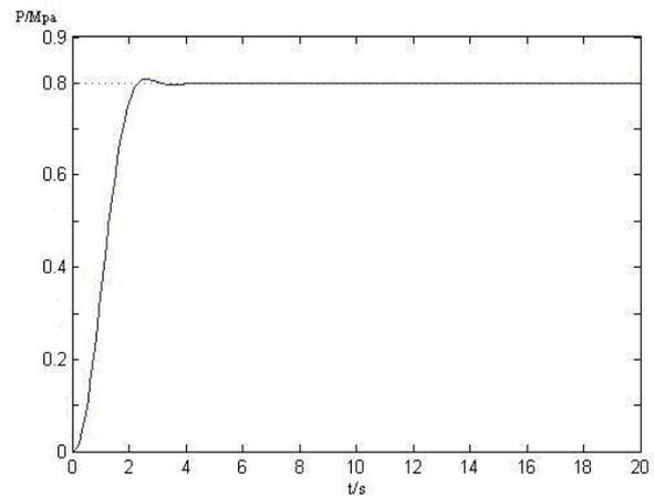
Figure 10. Simulation wave of fuzzy controller under step input
