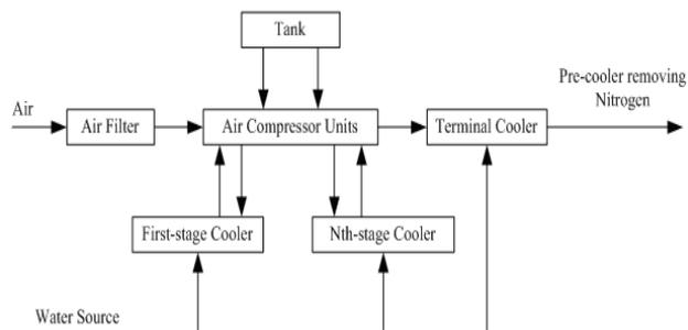
Figure 1. Process flow for air compressor system
