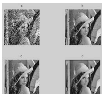
Figure 3. Restoration Results of Different Filters of Corrupted Lena Image with 30% Salt-and-pepper Noise
