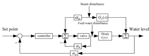
Figure 3. Drum level three impulses control system block diagram
