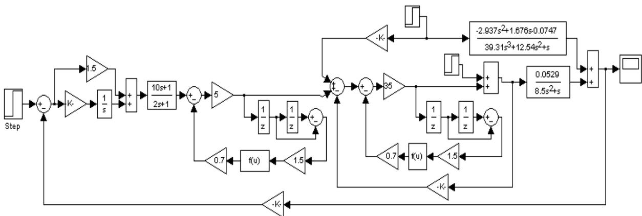
Figure 6 Immune incomplete differential PID -P cascade controller simulation diagram for feed water system
