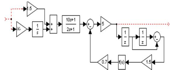
Figure 4 Immune incomplete differential PID main controller
