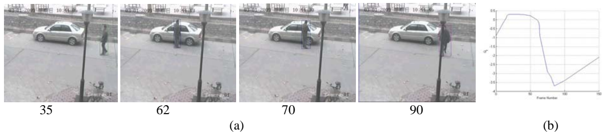
Figure 4. Example of anomaly detection in the entrance/exit area of an office building. (a) An abnormal activity where one people attempted to destroy the car parking the area. It resembles C3 in the early stage. (b) The activity was detected as an anomaly from Frame 62 till the end based on Q_t .
