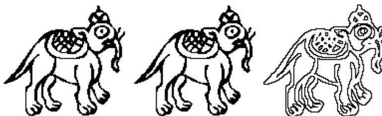
Figure 3. Contour extraction of Naxi pictograph. a. Normalized character. b. Character after binary processing. c. Character after contour extraction
