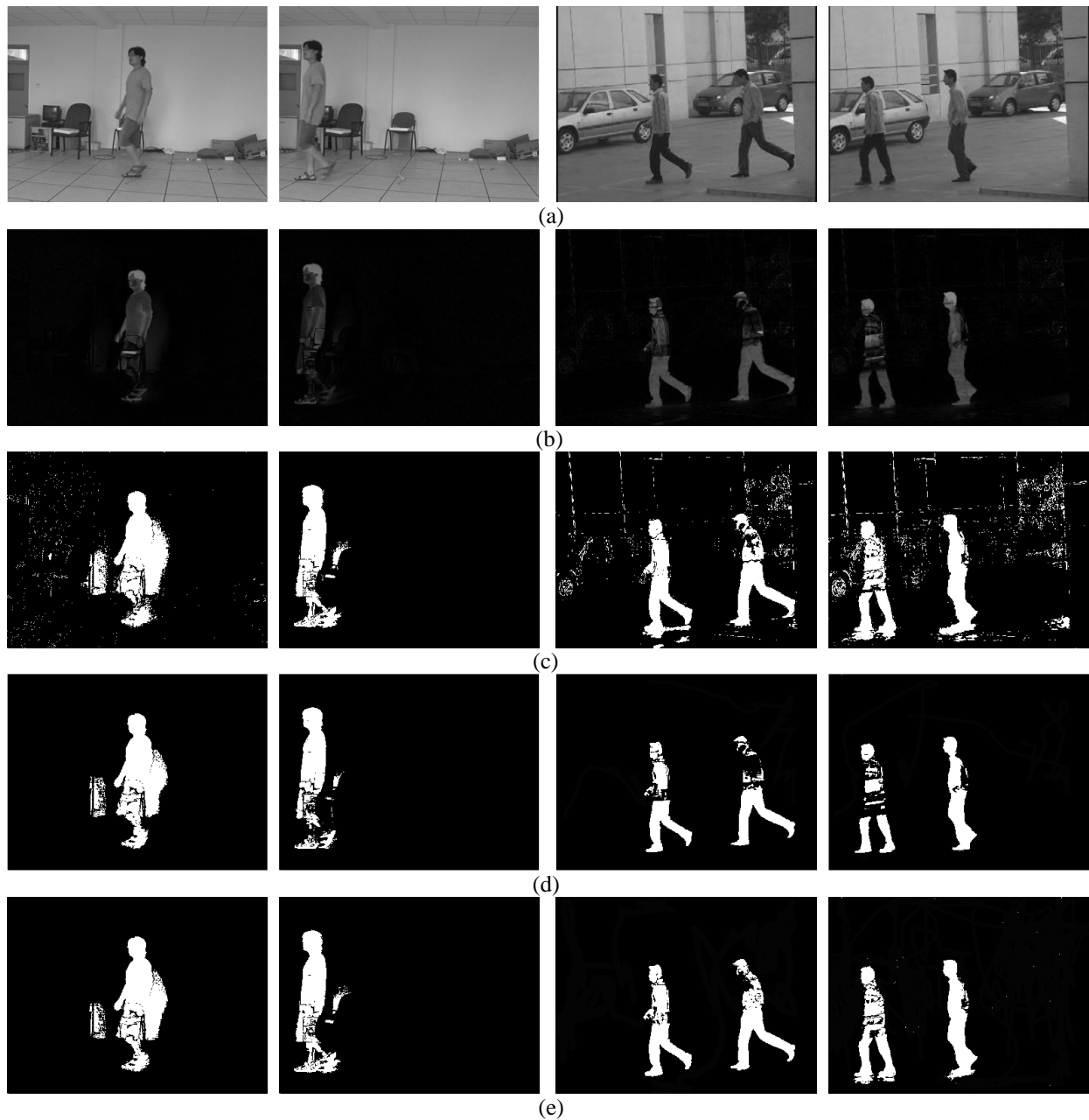
Figure 5. Detecting result comparison in two video sequences under indoor and outdoor circumstance (a) The original image under indoor and outdoor circumstance. (b) The gray difference image with background subtraction. (c) The detected result with fixed threshold 10. (d) The detected result with fixed threshold 15 and 25. (e) The detected result with optimal threshold.
