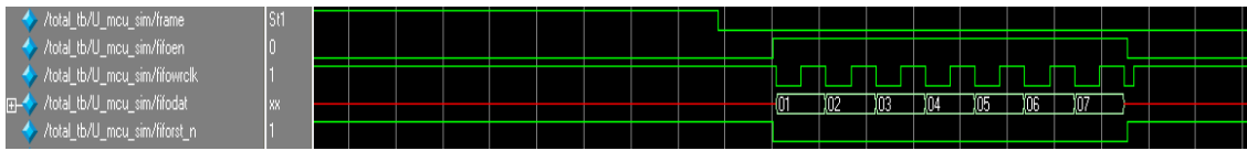
Figure 4. The writing process from the microprocessor to the FIFO
