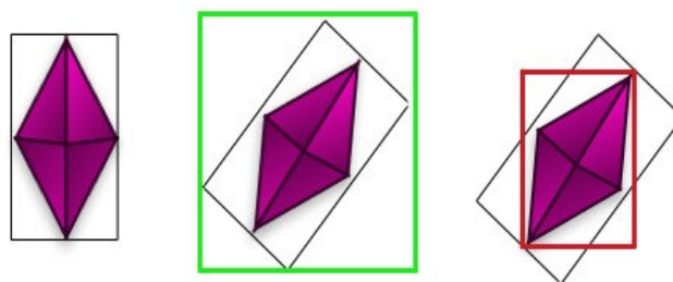
Figure 6 Updating Bounding box w.r.t. rotation, (a) AABB of the geometry, (b) Wrapping AABB around OBB, (c) Refitting of AABB
