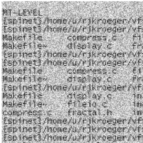
Figure 24. The Text image embedded with the color text watermark using the Daubechies 4 coefficient wavelet with speckle noise added - PSNR 16.65
