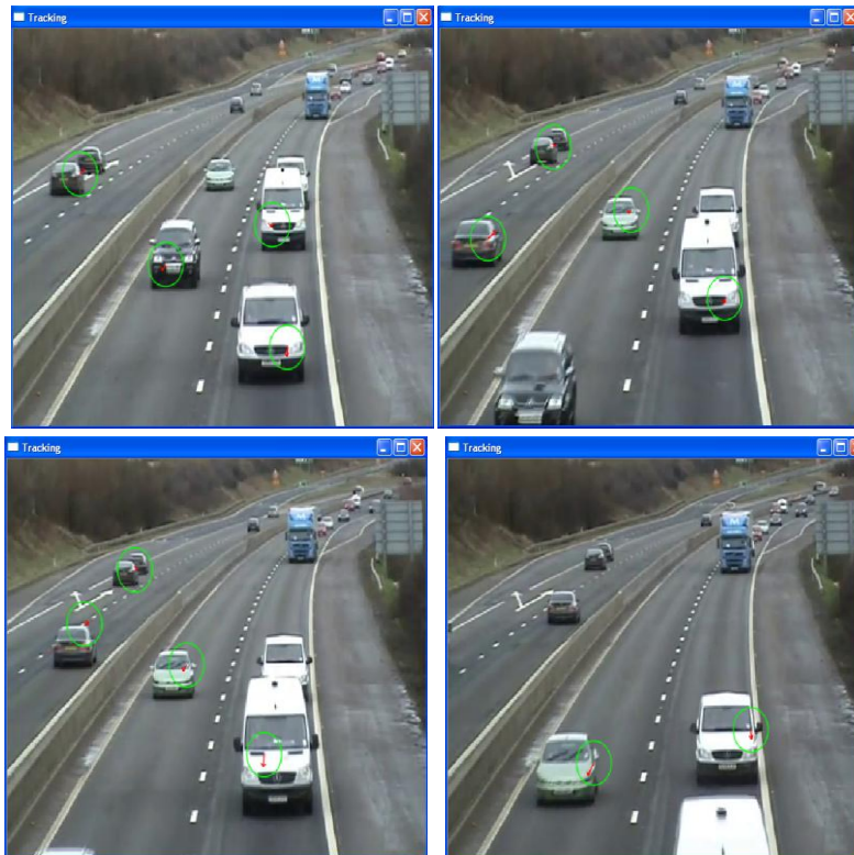
Fig. 4. Motion tracking and velocity estimation for many cars.
