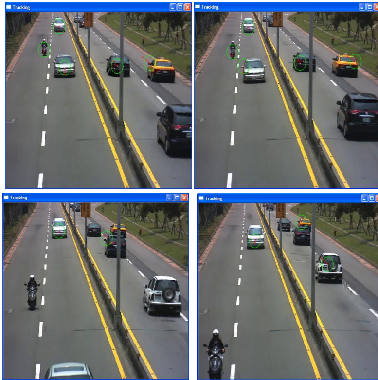
Fig. 3. Motion tracking and velocity estimation with occlusion effect at separator.
