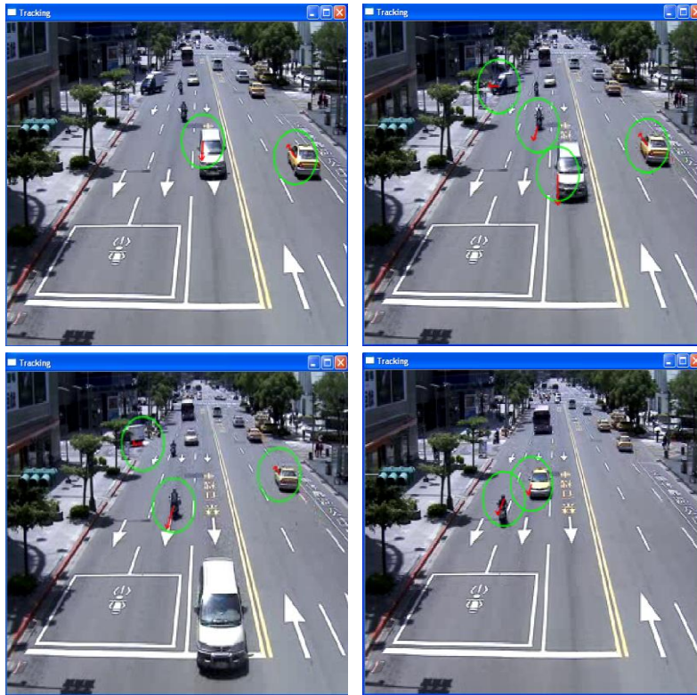
Fig. 5. Motion tracking and velocity estimation in the busy road.
